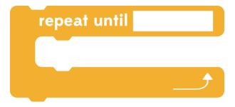
This block also allows to repeat, but only the light blue blocks fit in the rectangular area ("I touch colour?" or "I touch obstacle?").
